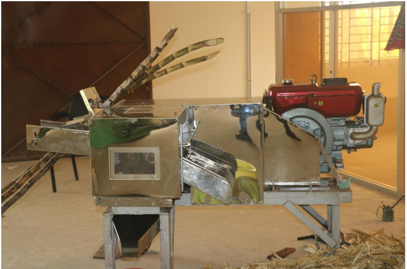
Pic.-1: Sugarcane Power crusher
