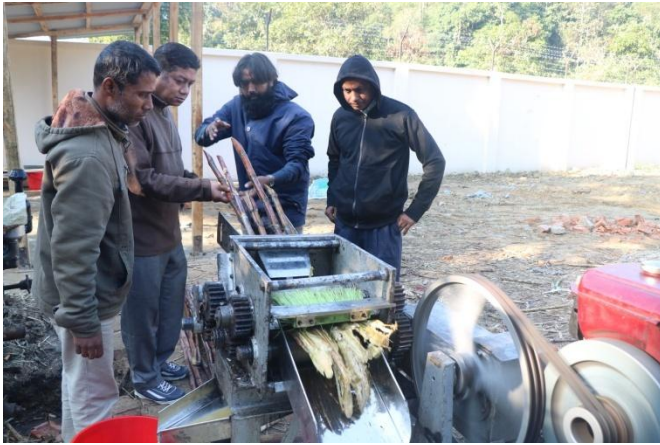
Pic.-2: Sugarcane Crushing capacity test at Bandarban
